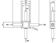
**ORDERING INFORMATION (PN)** FPDC=Polarization Beam Combiner; FPDS=Polarization Beam Splitter.
